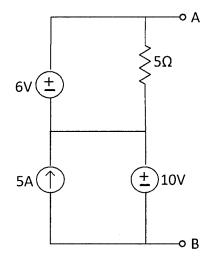
(6) Determine the current flowing in the following circuit.
